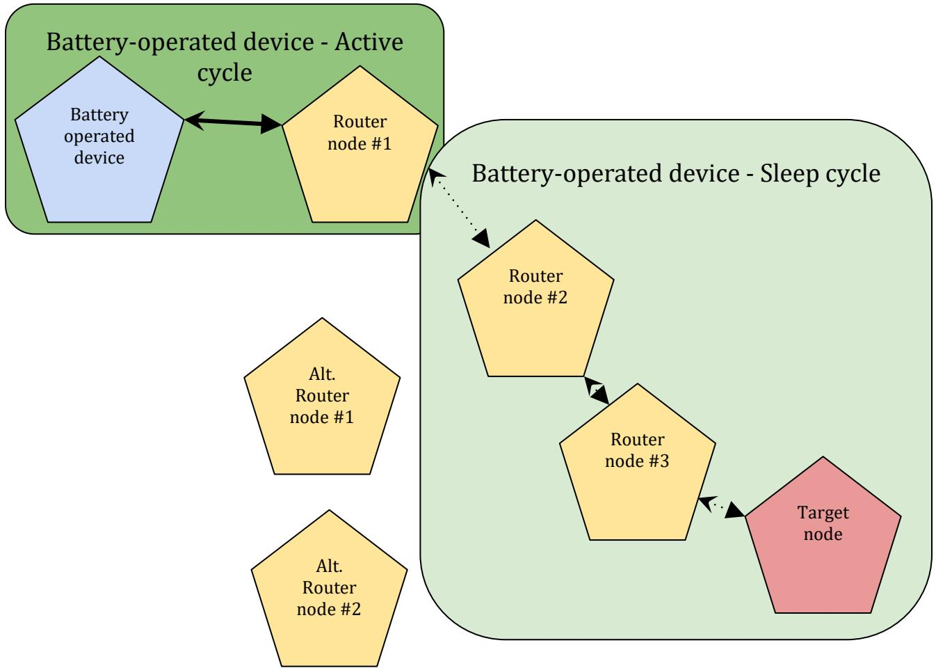
Figure 2: Routing of packet generated by a battery-operated device in a Thread network
