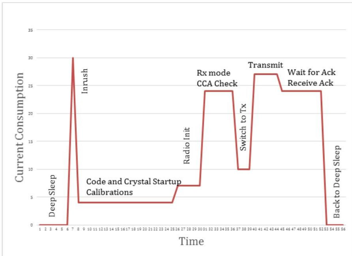
Figure 4: Typical wake-sleep cycle. In Y-axis the scale is in fraction of millampere, while in the X-axis is fraction of milliseconds.
