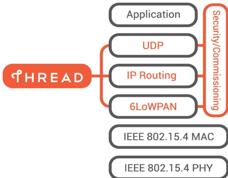
Figure 1: Thread protocol layering
