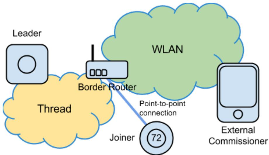
**Figure 2. Case 2: External Commissioner connected to the WLAN, Border Router is Joiner Router**
